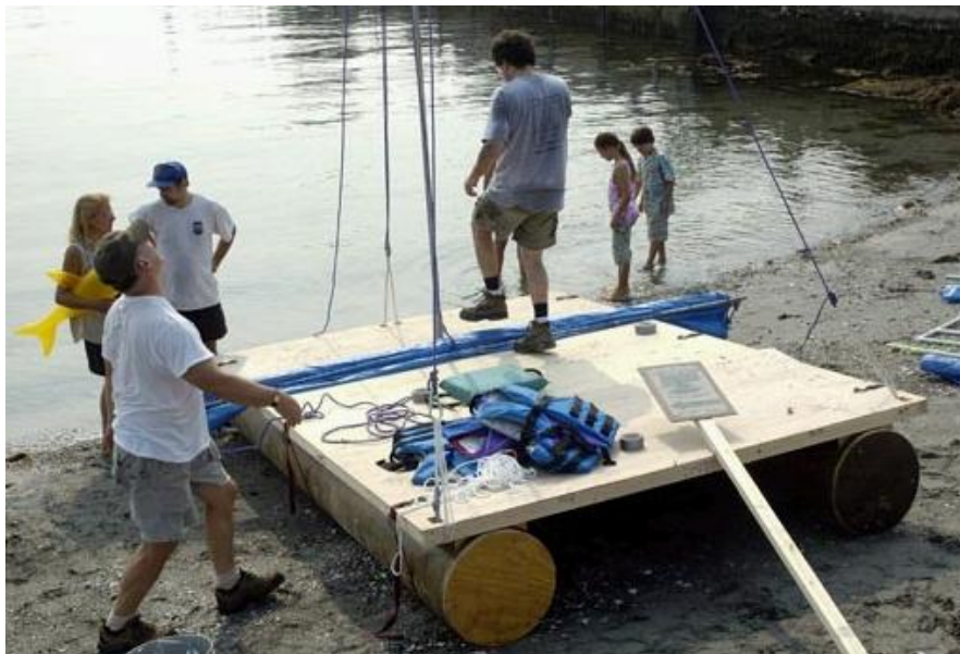
Here is a good deck design strapped to two Sonotubes.
